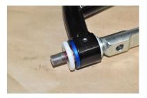
10. Install the steel outer washer and hex nut and grease fitting.
