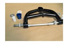
6. Next install the bushing on the other side. Use a suitable press tool such as described above for
