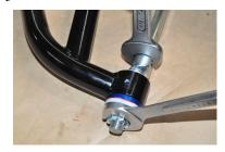
12. Once the torque is set, drill a cotter pin hole (1/8 inch) through the shaft.
