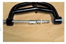
5. Next install the other side inner and outer thrust washers. This time install the steel washer first on the shaft and then the inner plastic washer.
