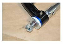
11. Adjust the preload on the bushing. The preload is adjusted similar to that of a wheel bearing. Run the hex down until the air gap between the thrust washers and bushing is gone. Seat the assembly like a wheel bearing and then back off the nut. Next run the nut till you have slight resistance and then tighten 1/8 of a turn or one flat on the nut.
