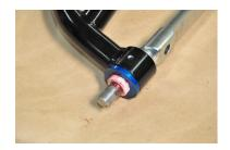
9. Install the outer thrust washer over the insert.
