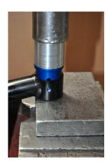
4. First: Slide the shaft through A-arm and install one small diameter steel thrust washer onto the shaft. Second: Place one small diameter white plastic thrust washer onto the shaft.
