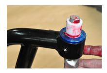
8. You may have to slightly tap the insert into the bushing. The insert will stick out past the bushing when it is seated.
