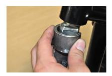
7. Next install the inserts into the bushing. Lubricate the inside of the bushing first and the place grease inside and out on the white insert.
