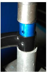
4. Next, grease the inside of the bushing housing and the plastic insert inside and out. Slide the steel pin into the insert after lubing.
