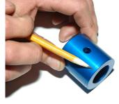
3. Line the hole in the bushing with the grease hole in the control arm. Press the bushing in until it is flush with the control arm housing
