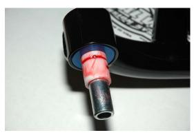
5. Install the plastic thrust washers on each side of the bushing.
