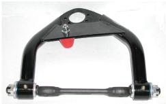
8. Use a 1/8-inch drill bit and drill a 1/8-inch hole through the shaft. You are going to cotter pin the hex nut so there will be no chance of the nut backing off. The hole should be drilled in the slot of the hex nut similar to that of a wheel bearing cotter pin setup. Cotter pin each end of the shaft before installing on the car.
