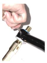
5. The next step is to install grease in the bushing housing and install the white plastic insert. The insert should have grease inside it as well. We use synthetic grease called NEO Part # GR-1. However any water resistant grease will work. Place the insert into the housing and slightly tap the insert into the housing. Both sides of the control can be done.
