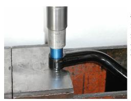
Slide the shaft all the way through the control arm. Take a blue bushing housing and press in into the other side of the upper arm. If you will notice in the picture we use a (V) block for pressing in the bushing. The shaft and thrust washers are in the (V) area of the block.
