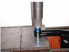
Note: The hole in the bushing should be in a position so it is straight up when the arm is placed on the car.
