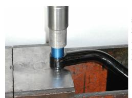
Slide the shaft all the way through the control arm. Take a blue bushing housing and press in into the other side of the upper arm. If you will notice in the picture we use a (V) block for pressing in the bushing. The shaft and thrust washers are in the (V) area of the block.
