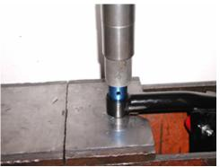
Note: The hole in the bushing should be in a position so it is straight up when the arm is placed on the car.
