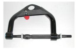
First: slide one small steel thrust washer onto the shaft.
