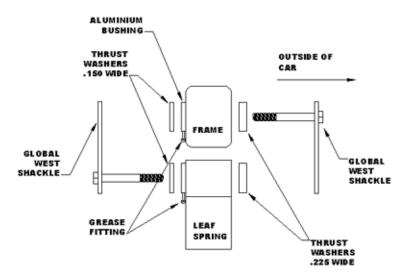
Note: Shackle halves are installed as follows: The bolt on the outboard shackle half goes through the frame and the bolt on the inboard shackle half goes through the spring eyelet bushing.
