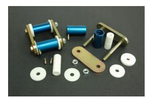
the shackle up from moving and create a harsh ride. Set properly the bushings will be unnoticed and give you long service. You do not need the vehicle on the ground to torque the bushings.
