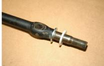
washers. Install the thrust washers on both side of the shaft.
