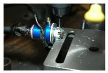
12. Install a cotter pin after drilling.
