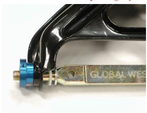
Slide the small steel inner thrust washer onto the shaft first, followed by the smaller delrin plastic washer-- one on each end of the shaft. (See diagram above). Next push the delrin (white) plastic inserts out of your new bushings. The bushings will install easier with the inserts out of the housings.
