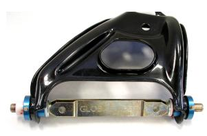
4. Press the aluminum bushings into the control arm, making sure that the hole for the grease zerk fitting is positioned in such a way that you will be able to access the zerk for lubrication purposes once the control arms are installed on the vehicle!
