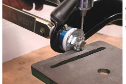
to cotter pin the hex nut so there will be no chance of the nut backing off. The hole should be drilled in the slot of the hex nut similar to that of a wheel bearing cotter pin setup. Cotter pin each end of the shaft before installing on the car.
