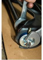
that of a wheel bearing cotter pin setup. Cotter pin each end of the shaft before installing on the car.
